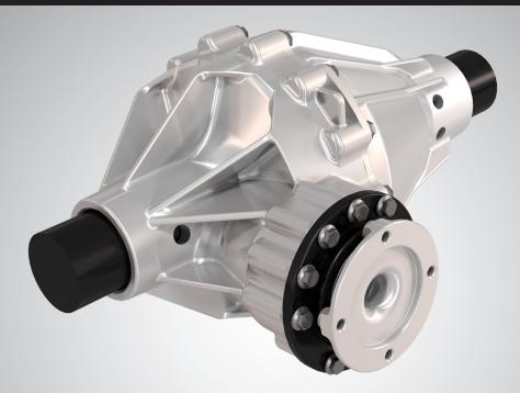
Mass Reduction — QUANTUM<sup>™</sup> axles are about 35% lighter than a typical axle.
