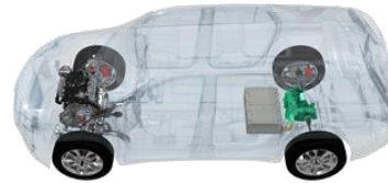
P4 SPLIT AXLE HYBRID ARCHITECTURE
